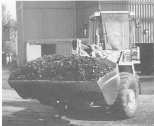
1995: Tire-derived fuel successfully burned in Boilers #7 and #8. Shown above, a front-end loader moves the tire-derived-fuel mixture to the Power Plant.
